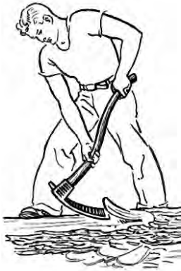
Using an Adze on timber
